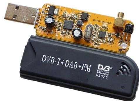
*Figure 2 – The RTL-SDR receiver. The plastic shell of the dongle has been removed so that the components can be seen*
